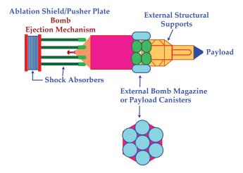
Figure 2 — Nuclear Pulse Vehicle<sup>13</sup>
