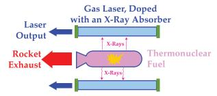
Figure 3 — Schematic of a thermonuclear rocket-laser drive propulsion system (adapted)<sup>19</sup>
